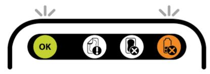
The pump runs on two AA alkaline batteries. If the "Low Battery" light starts to flash at the same time as the green "OK" light, it means there is less than 24 hours of charge left, and you should change the batteries.
